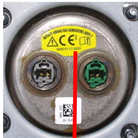
Counterfeit airbag looks nearly identical to the genuine airbag
